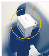
Press release button to remove connector
